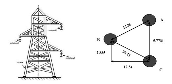
Vertical distance between two conductors (y) = 5.77 m = DacHorizontal distance between two conductors = 12.54 m Applying Pythagoras theorem,
